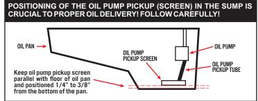
pan baffles, etc.). If no adjustments are required, remove the oil pan and permanently install oil pump. Measure the distance between the oil pump pickup screen and the pan floor. The clearance MUST be between 1/4" - 3/8" with the Hamburger's oil pan gasket installed. If you are using a high volume pump, you may need to modify the pickup.
